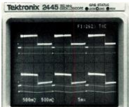
In many cases a.c. coupling is desired, but the resulting waveform tilt makes measurements difficult. Noticeable waveform tilt is present on the three fields of live video displayed on the lower trace. On the upper trace, the TV (backporch) clamp removes this tilt from the waveform.
