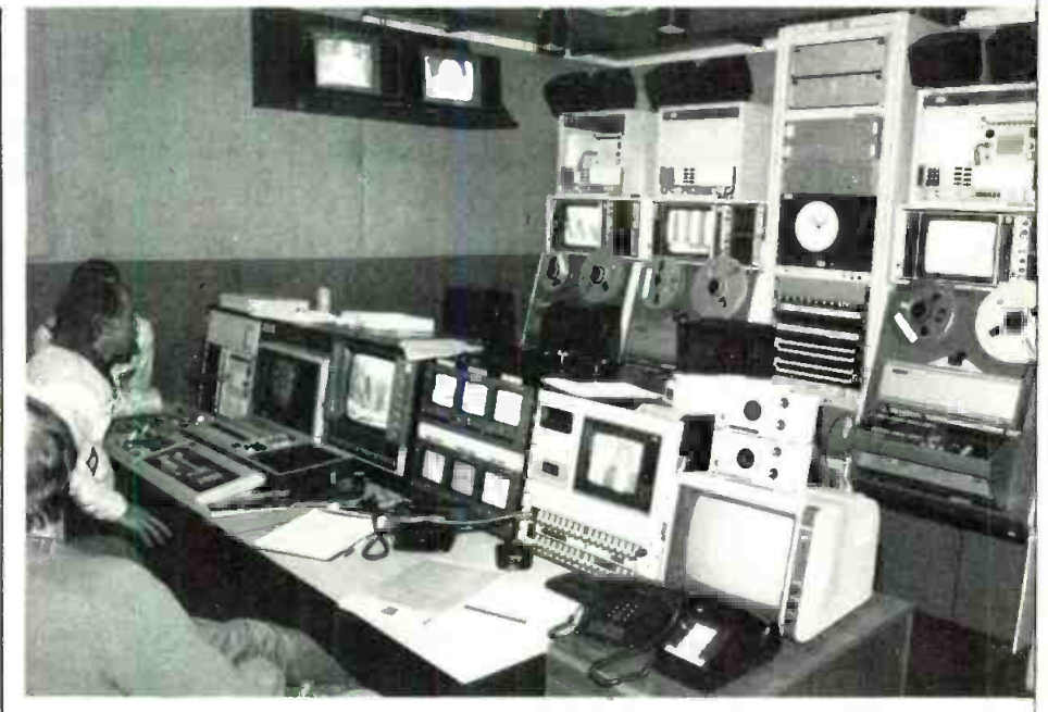
▲ Control Room A. The main control room of ABC's broadcast center in Sarajevo, Yugoslavia. At left (lower level) is executive producer Roone Arledge's desk. Production switcher has 22 inputs. To right on lower level is main on-air audio mixing area. On second level, to right, is Julie Barnathan's command desk.
