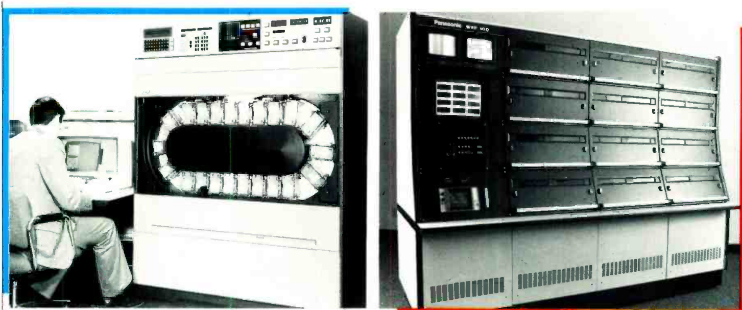
The old and the new. At left, RCA's TCR 100, developed in the late 1960s. At right, Panasonic's new M-format MVP-100 MERPS.
