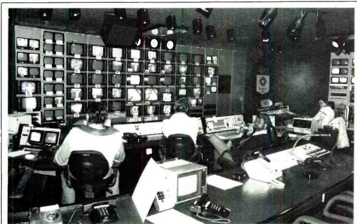
▲ Control Room A. The main control room of ABC's broadcast center in Sarajevo, Yugoslavia. At left (lower level) is executive producer Roone Arledge's desk. Production switcher has 22 inputs. To right on lower level is main on-air audio mixing area. On second level, to right, is Julie Barnathan's command desk.
